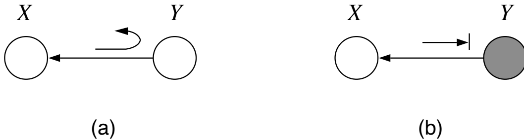
Figure 2.13: The rules for this case follow from the rules in Figure 2.10. (a) When the ball arrives at an unshaded node, the ball “passes through,” which effectively means that it bounces back. (b) When the ball arrives at a shaded node, the ball is blocked.
