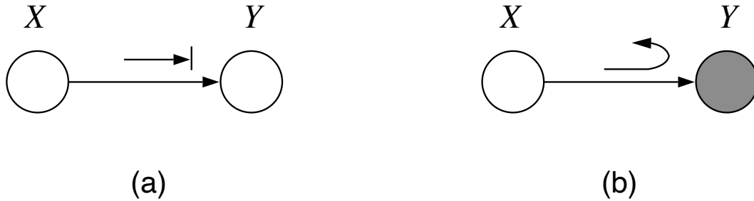
Figure 2.12: The rules for this case follow from the rules in Figure 2.11. (a) When the ball arrives at an unshaded node, the ball is blocked. (b) When the ball arrives at a shaded node, the ball “passes through,” which effectively means that it bounces back.
